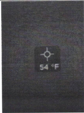
Dining room supply air temperature was 54°
