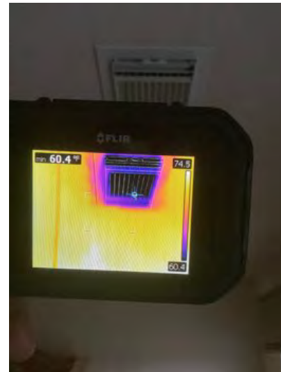
Second floor back left bedroom temperature reading. 60.4 degrees noted. Observational an informational purpose only.
