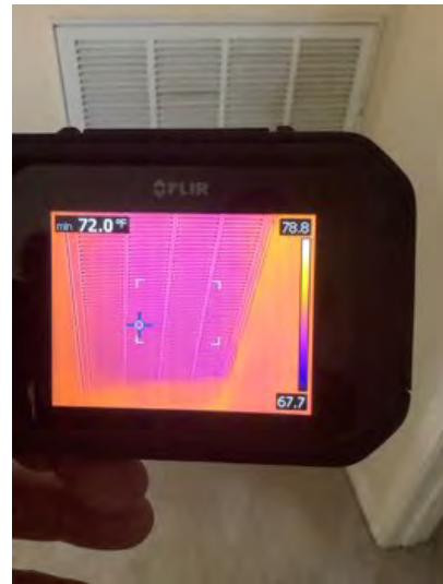
72° temperature reading on second floor return vent in wall located at top of stairs noted. Observational an informational purposes only.
