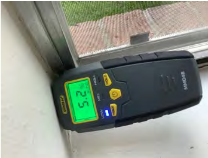
Moisture readings on window in master bedroom was a normal range observational an informational purposes only.
