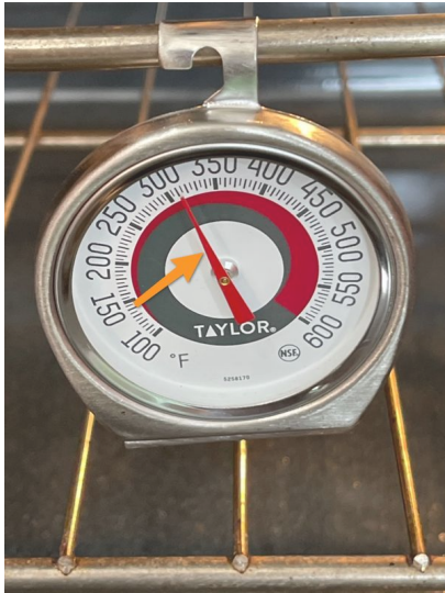
Oven set at 350 degrees, temp readings 310 degrees
