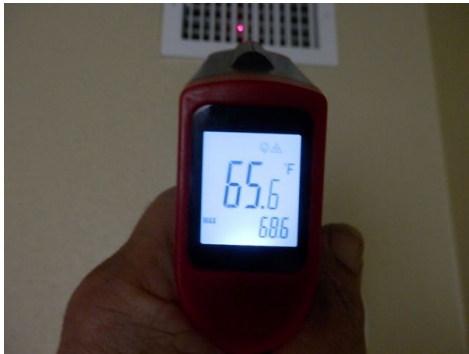
checking the cooling output - one outside a/c appeared to be dated 2008 with R-22 coolant
