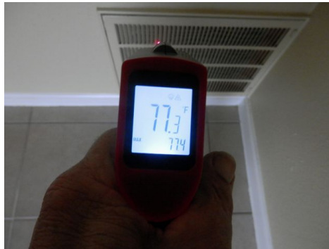
checking the cooling output - one outside a/c appeared to be dated 2008 with R-22 coolant
