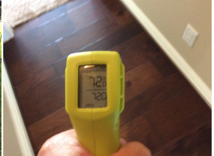
Downstairs cooling return temperature 72°
