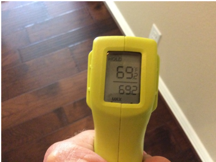
Downstairs heating return temperature 69°
