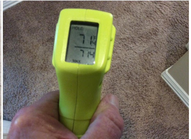
Upstairs cooling return temperature 71°
