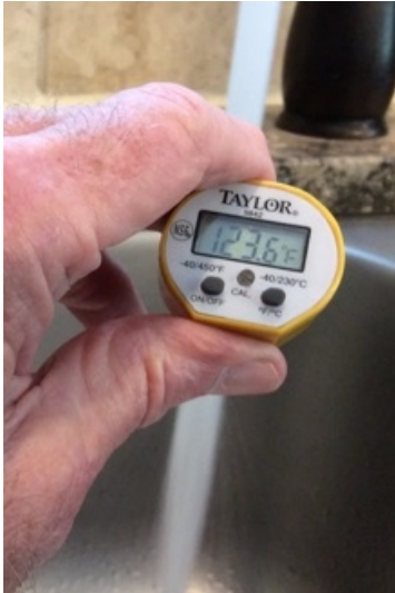
Hot water temperature measured at the kitchen sink was 123.6°
