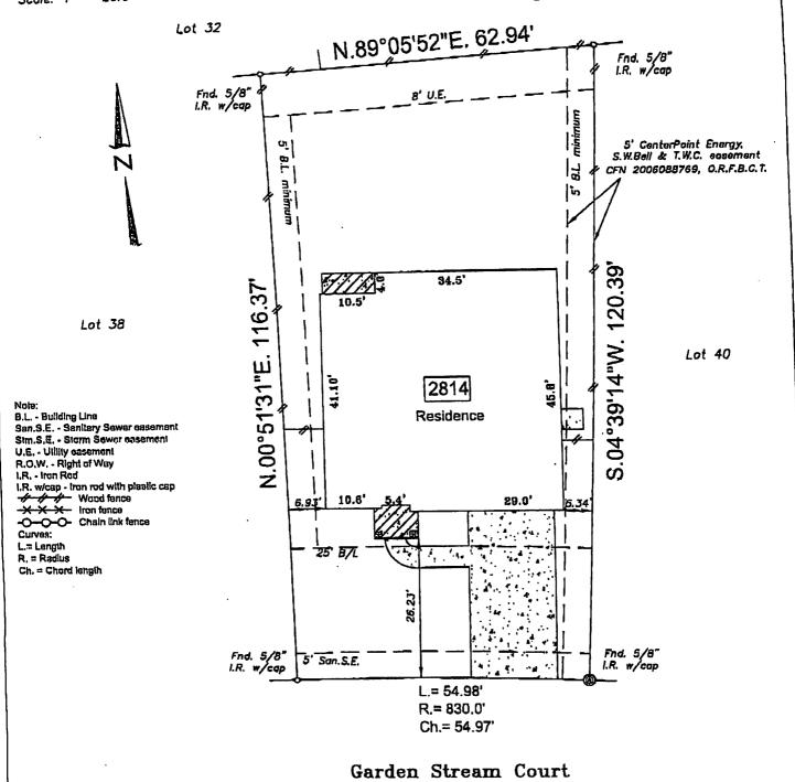
In accordance with FEMA Community Panel #'s 48157C0210—J & 48157C0230—J revised January 3, 1997 this property lies in Zone "X" & shaded Zone "X". (per recorded plot) inherent inaccuracies of FEMA or flood control maps preclude a surveyor from certifying to the accuracy of potential flooding locations based on such maps.
