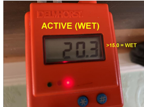
Moisture meter reading of floor in the foyer.
