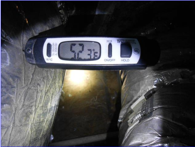
B. Item 7(Picture) View of the second floor cooling system measured exit air temperature at the evaporator.
