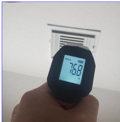
A. Item 2(Picture) Heater not heating after being on for approximately 15 minutes
