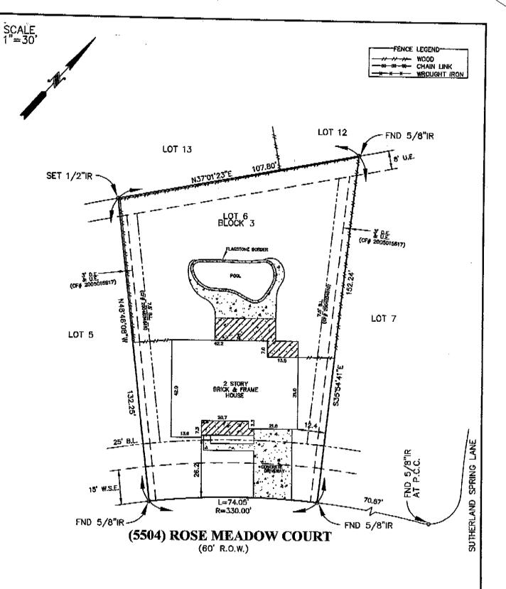
Note: All bearings shown hereon are based on the record plat indicated below. Note: Restrictive covenants as recorded in V-24, P-6-7 BCPR and CF#s 97-032630, 01-057355, 02-030661, 2004026391, 2004034618 and 2005015617 ORBC.
