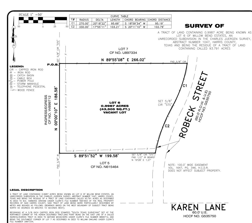
1. BASIS OF BEARING IS THE WEST BOUNDARY LINE OF SUBJECT TRACT BEING N 00°00'10" W. 2. SURVEYOR DID NOT ABSTRACT PROPERTY. SURVEY BASED ON LEGAL DESCRIPTIONS SUPPLIED BY TITLE COMPANY, SURVEY AS SHOWN AND LEGAL DESCRIPTION ARE PER AN ON THE GROUND SURVEY. EASEMENTS, BUILDING LINES, ETC., SHOWN ARE AS IDENTIFIED BY GF NO. 2619188-HO90 OF FIRST AMERICAN TITLE GUARANTY COMPANY. EFFECTIVE DATE: APRIL 01, 2021
