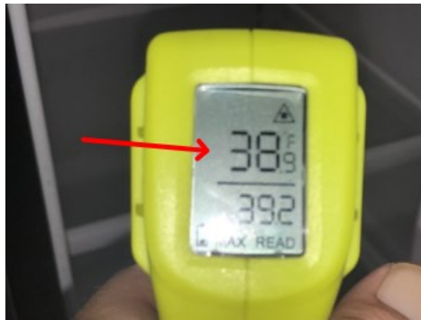
Refrigerator cool temperature
