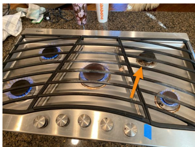
Back right burner did not ignite on its own
