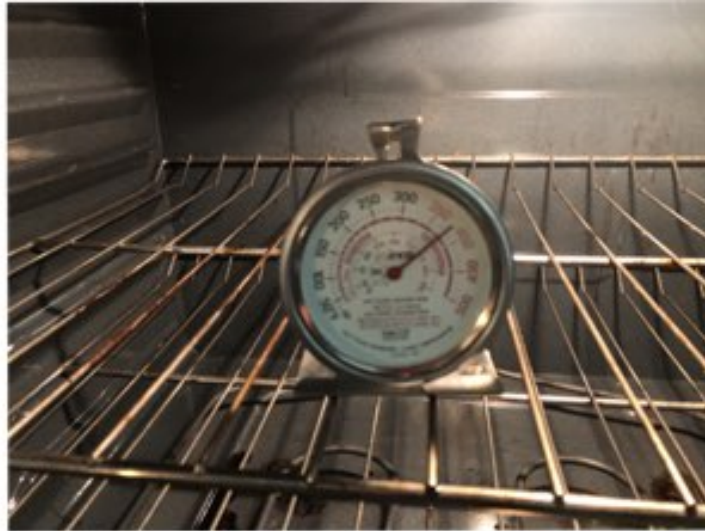
The oven is running about 25 degrees hotter than the setting of 350 degrees.
