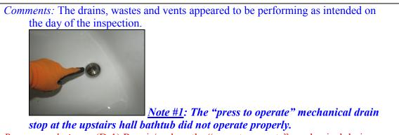
*Recommendations:* (D-1) Repair/replace the "press to operate" mechanical drain stop at the upstairs hall bathtub.
