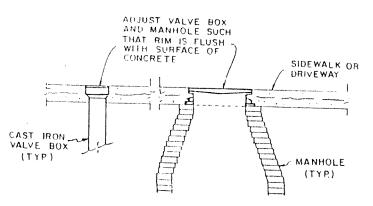
WATER VALVE BOX AND MANHOLE IN SIDEWALK OR DRIVEWAY
