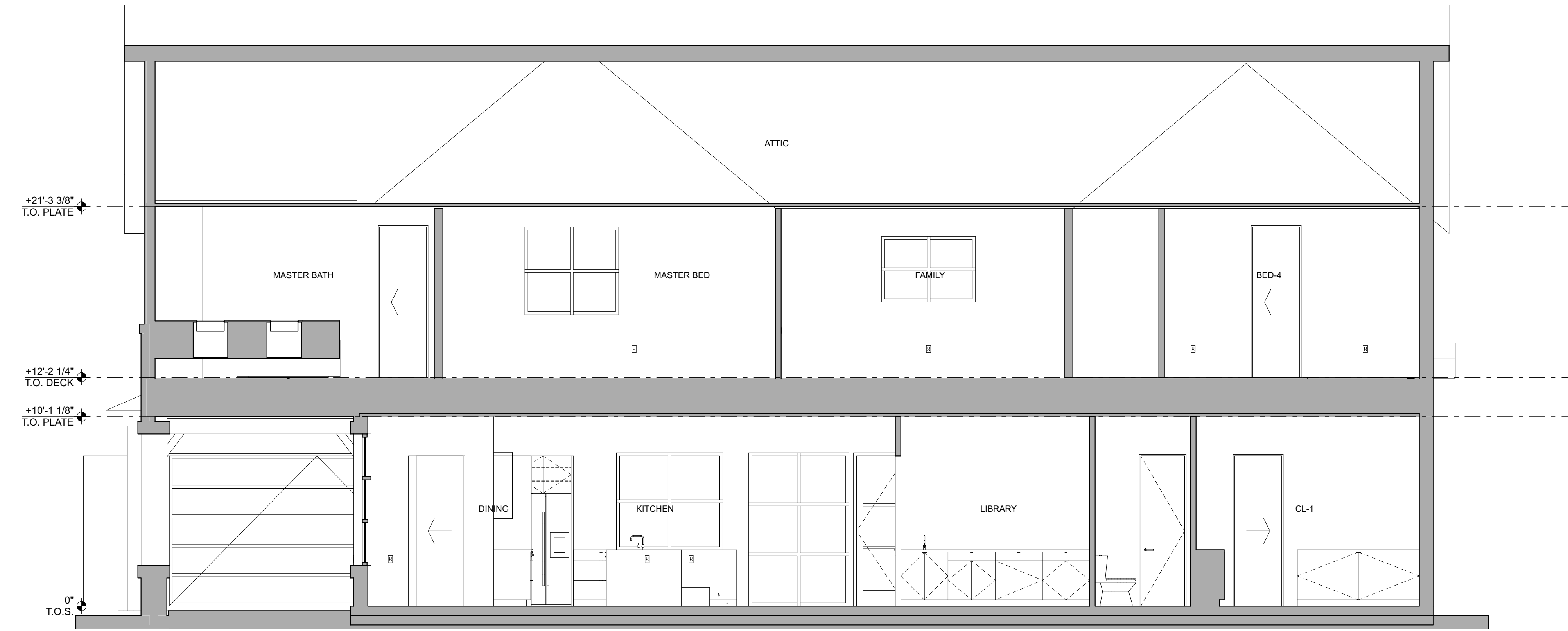
E-W BUILDING SECTION 02 SCALE: 1/4" = 1'-0"
