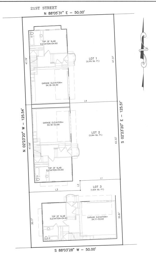
NOTE: FLOOR PLAN SHOWN HEREON PER ARCHITECTURAL DRAWNGS FOR REFERENCE ONLY, ONLY WOOD FORMS EXIST AT THE TIME OF THIS SURVEY.
