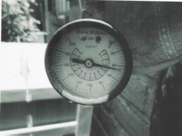
The water pressure to the house at the time of the inspection was checked with a pressure gauge at the hose bibb nearest the shut off valve, and the pressure was observed to be 50 psi.
