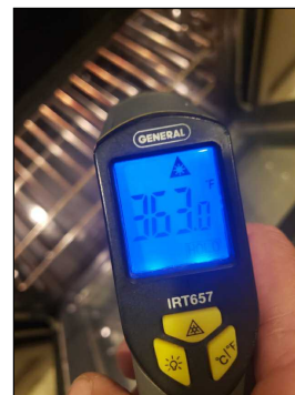
Oven operated within the 350 +/- 25 degrees F range
