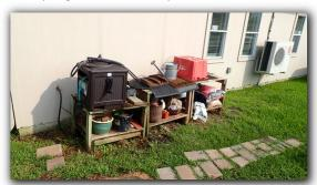
Soil grade and drainage patterns around some areas of house do not appear to properly direct water away from foundation to aid in controlling runoff water and could cause differential movement of the foundation or water penetration during heavy rains.
