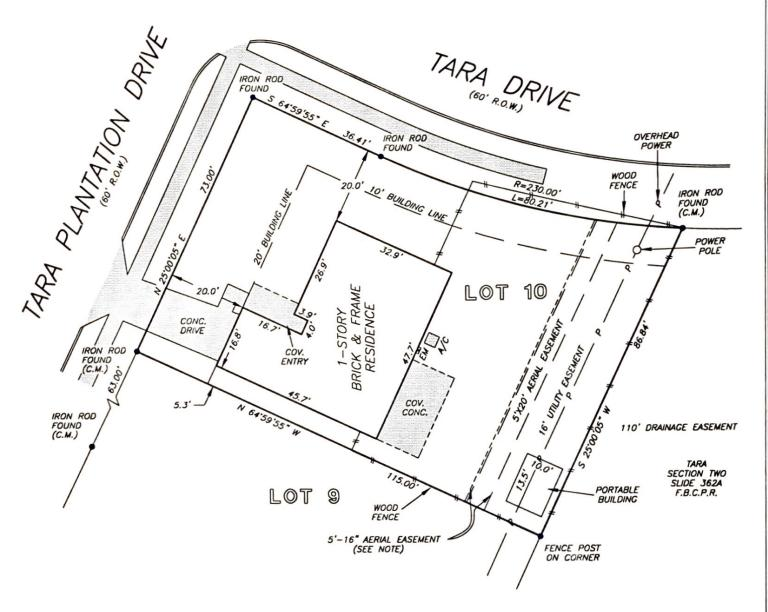
NOTE: AN UNOBSTRUCTED AERIAL EASEMENT 5'-6" IN WIDTH EXTENDING UPWARD FROM AN INCLINED PLANE BEGINNING AT A HEIGHT OF 16'-3" ABOVE THE GROUND ADJACENT TO THE 16' UTILITY EASEMENT AND CONTINUES OUTWARD TO A HEIGHT OF 18'-6" AS PER INSTRUMENT RECORDED IN VOL. 810, PG. 45, F.B.C.D.R.
