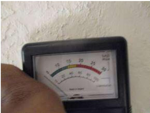
Water stains were observed on the walls. The stains were checked with a moisture meter, and no higher than normal moisture readings were found at the time of the inspection. The source of the water stains could not be determined at the time of the inspection, and further investigation is recommended with the homeowner and/or a service company.
