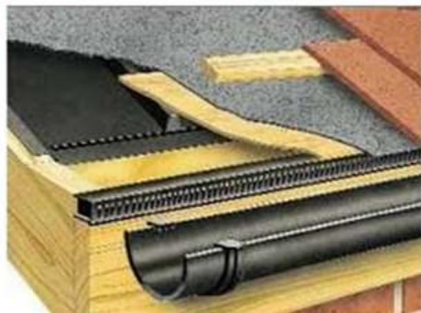
The ventilation for the attic included continuous ridge vents and continuous soffit vents.
