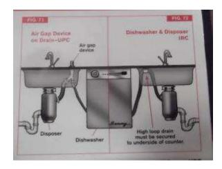
The drain line under the sink was looped up so that the top of the loop was higher than the point where the drain line connected to the disposal. This will help to prevent garbage from running down the drain line into the dishwasher.
