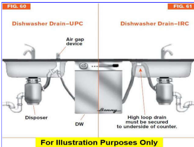
A. Item 5(Picture) Air Gap/High Loop
