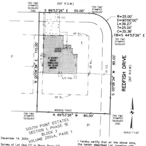
Survey of Lot One (1) in Block Three (3) of SOUTH POINT ESTATES, SECTION ONE (1), PHASE 1B, a Subdivision in Galveston County, Texas, according to the map or plat thereof recorded in Volume 2004A, Page 1, of the Map Records in the Office of the County Clerk of Galveston County,
