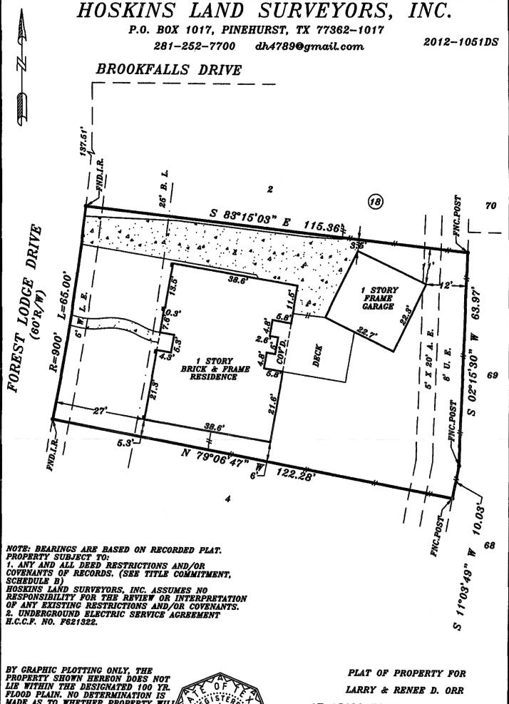
BY GRAPHIC PLOTTING ONLY, THE PROPERTY SHOWN HEREON DOES NOT LIB WITHIN THE DESIGNATED 100 YR. FLOOD PLAIN. NO DETERMINATION IS MADE AS TO WHETHER PROPERTY WILL OR WILL NOT ACTUALLY FLOOD. FIRM PANEL NO. 48201C 0430L ZONE: "X" DATE: 06-18-07
