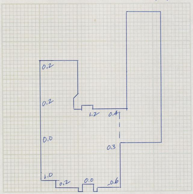
Foundation elevation readings vary approximately <u>l.8</u>" from high to low measurements.
