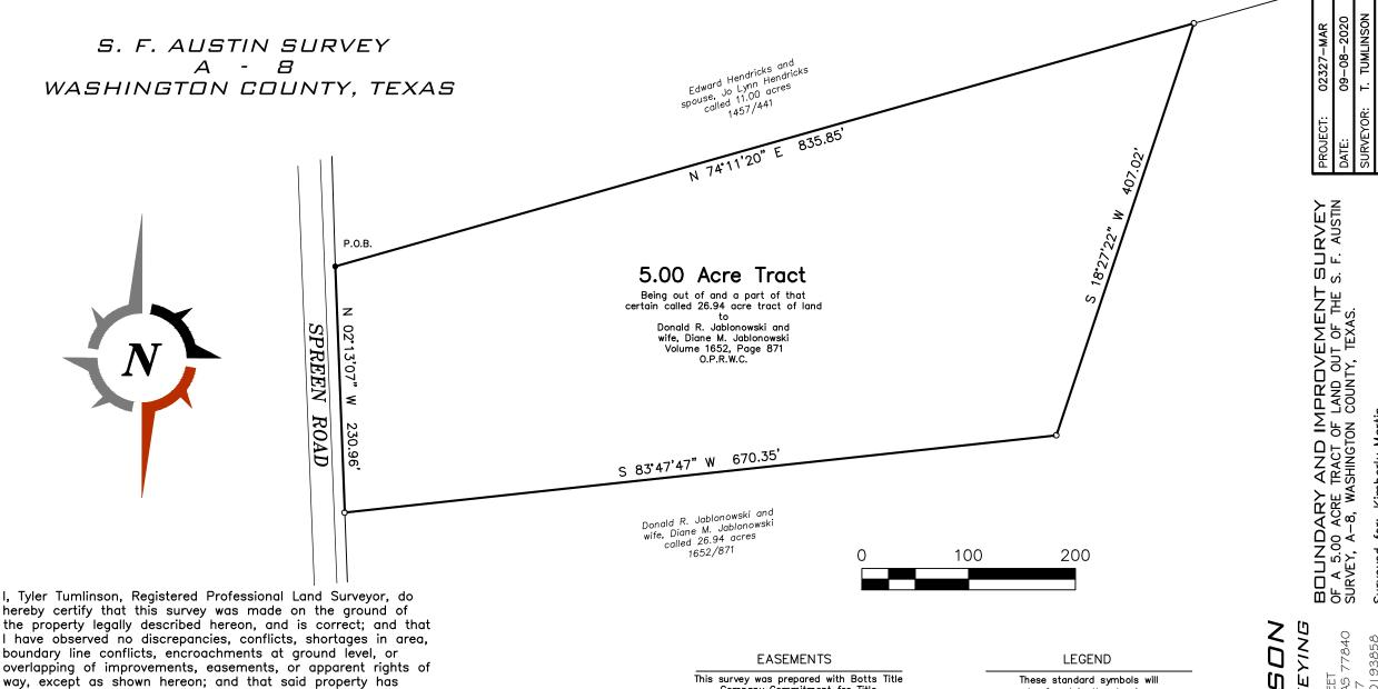
All bearings and distances are based on State Plane Coordinate System, Texas Central Zone, NAD 1983.
