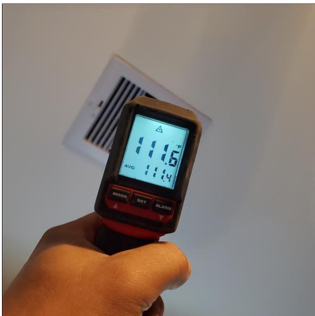
A. Item 2(Picture) Heating system providing warm air.
