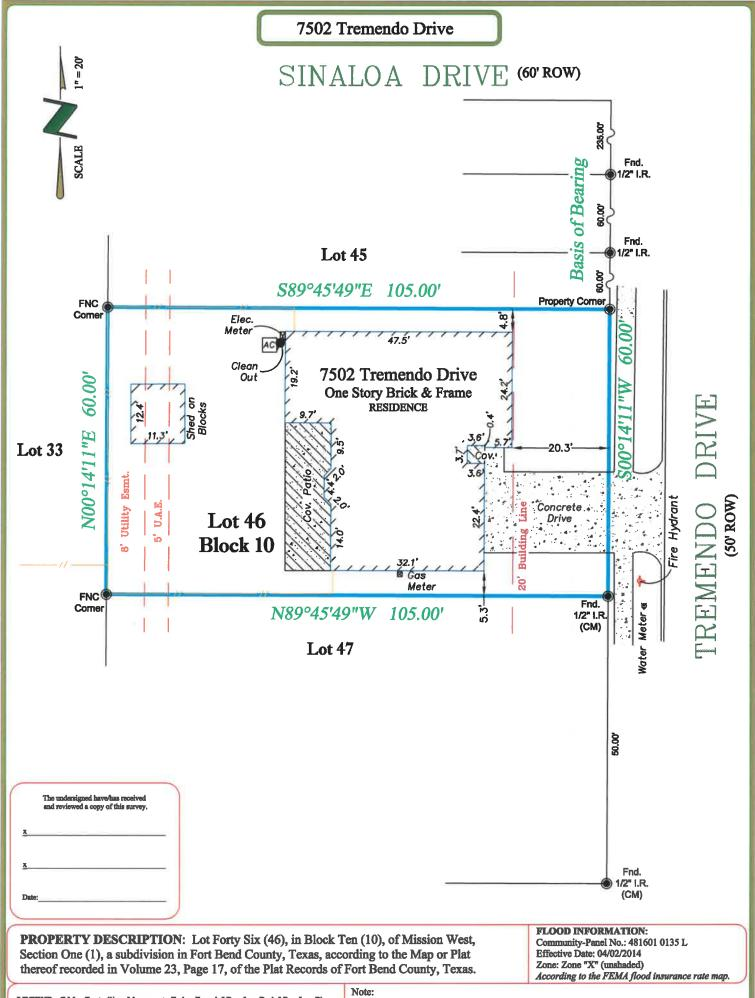
LEGEND - C.M.= Controlling Monument; Fnd. = Found; I.R. = Iron Rod; I.P.= Iron Pip OHE=Overhead Electric. I.R.S.= Set Iron Rods 5/8" diameter with yellow cap stamped "Arthur Surveying Company". centerline @ (overhead electric) -
