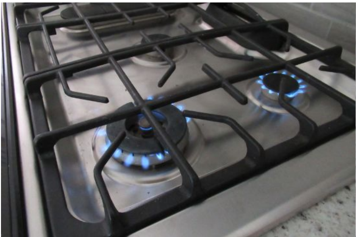
The burners: not all flames came on
