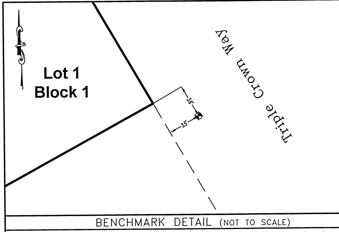
The site benchmark consists of a three inch brass disk in a six inch concrete column, & stamped "OKF2" Elev. = 196.23 based on NAVD88 Geoid 12B.
