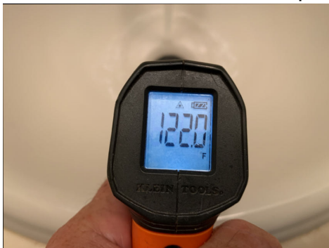
Hot water temperature: Scalding
