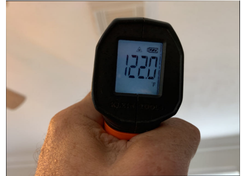
1st floor hot air temperature
