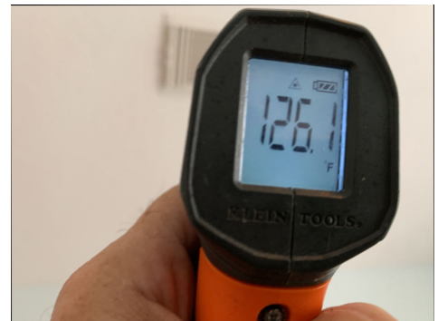
2nd floor hot air temperature
