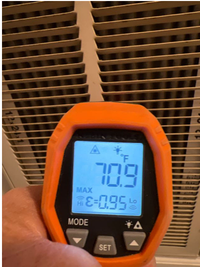
Air temperature measured at return air vent.
