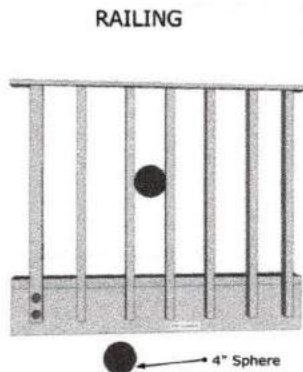
Example of Proper Railing Construction
