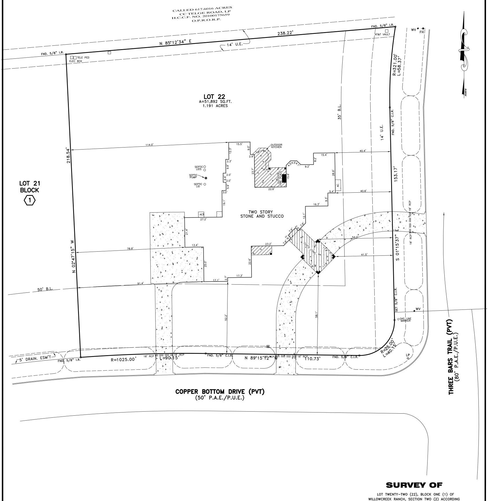
1. BEARING BASIS IS NORTH R.O.W. LINE OF COPPER BOTTOM DRIVE BEING NORTH 89 DEGREES 15 MINUTES 12 SECONDS WEST.
