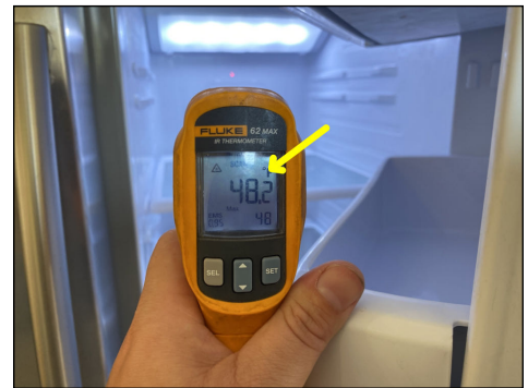
Refrigerator temp second floor kitchen.
