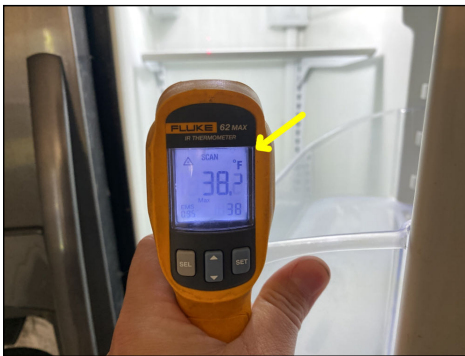
First floor kitchen refrigerator temp.
