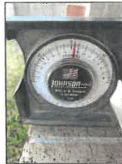
Rear, brick window sill sloped 5°
