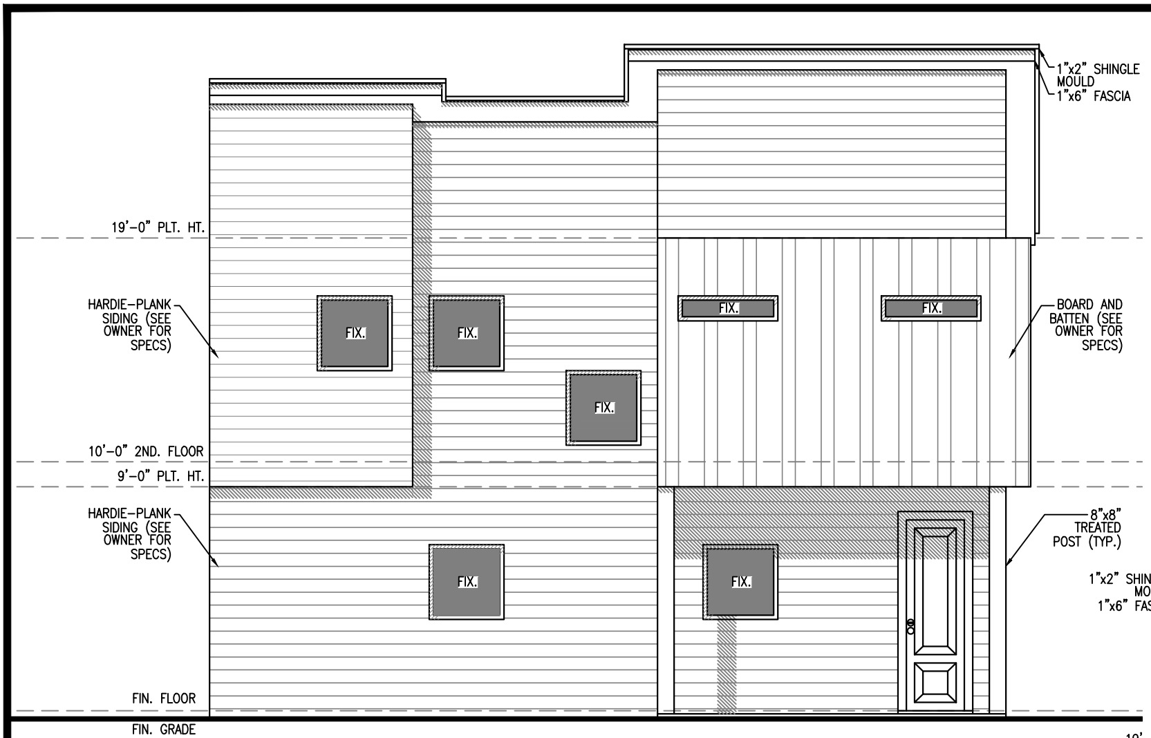
EXTERIOR ELEVATION FRONT SCALE: 3/16"=1'-0"
