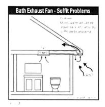
34. Observed exhaust vents routed to soffit. The problem is moist warm air can be drawn back into the attic by soffit vents and wind. Recommend rerouting the ducts to exhaust at a higher vent.
