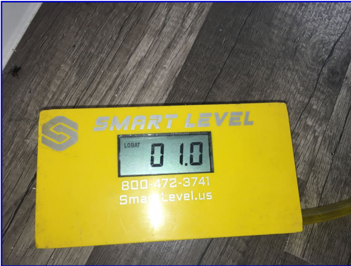
Foundation Elevation: Front right corner of home
