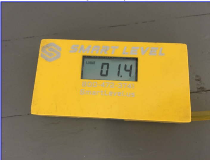
Foundation Elevation: Back left corner of home
