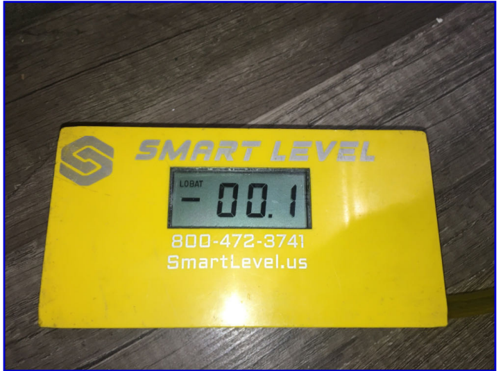
Foundation Elevation: Back center of home
