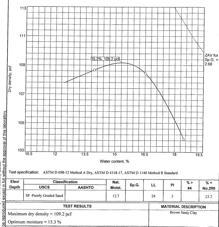
Test specification: ASTM D 698-12 Method A Dry, ASTM D 4318-17, ASTM D 1140 Method B Standard
