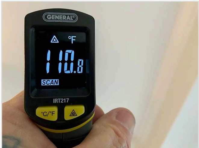
Supply air temperature 110.8°
