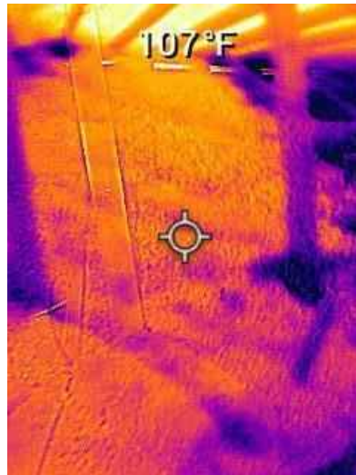
The insulation is sufficient in most areas of the attic
