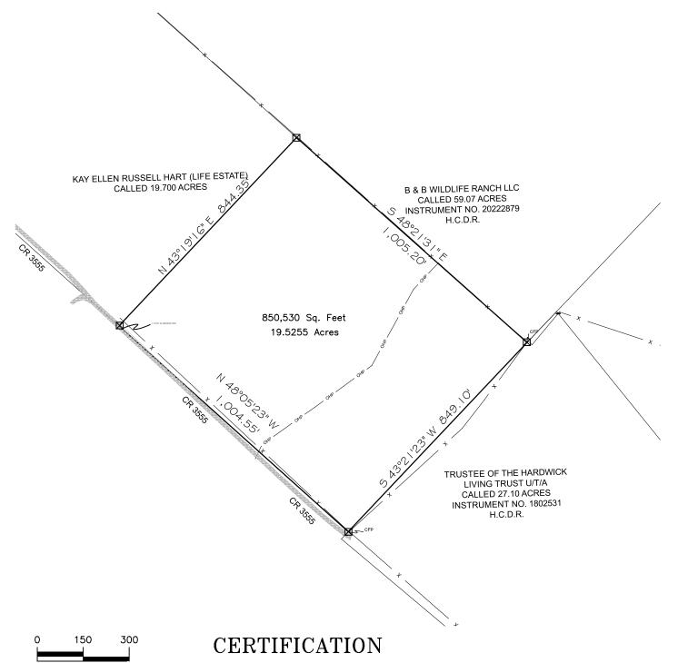
Basis of Bearings for this Survey is Grid North from GPS Observation TEXAS CENTRAL 4203 NAD83
