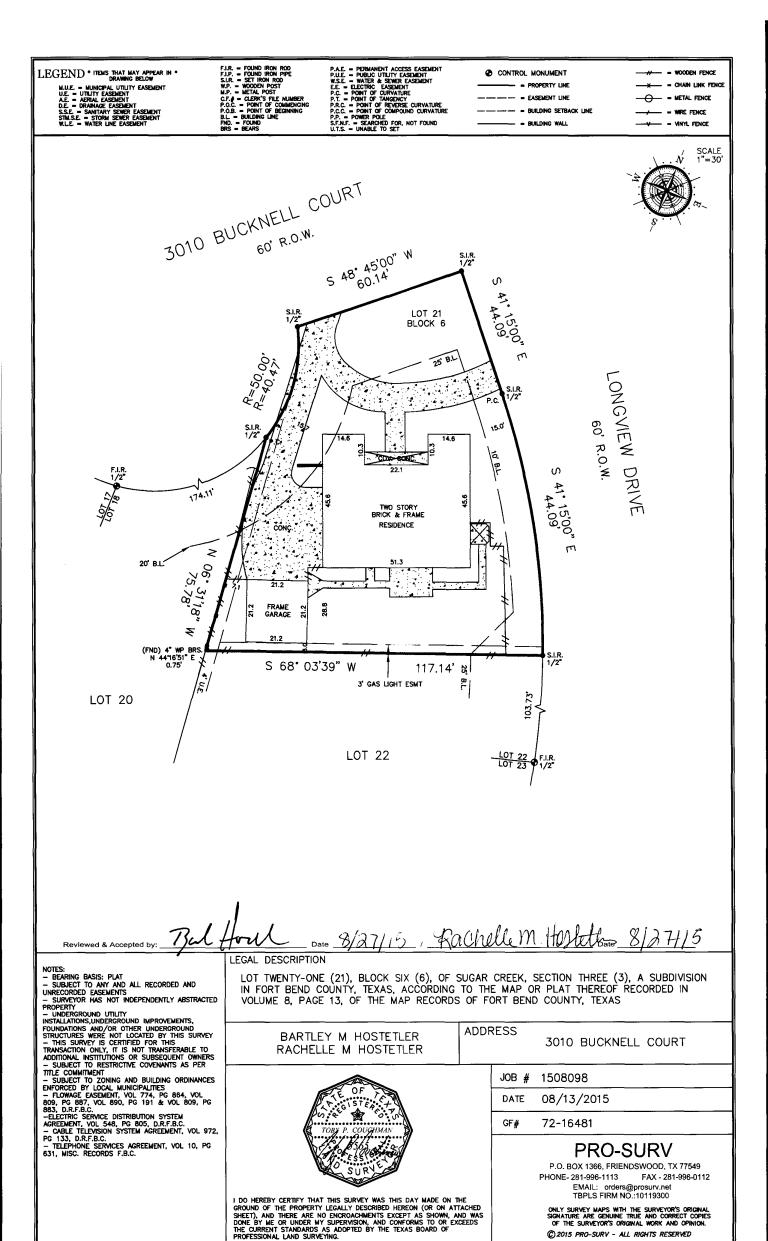
LEGEND \* ITEMS THAT MAY APPEAR IN \* CONTROL MONUMENT - WOODEN FENCE - PROPERTY LINE - = CHAIN LINK FENCE ------ = EASEMENT LINE - = METAL FENCE - WIRE FENCE - = BUILDING WALL 3010 BUCKNELL COURT S 48° 45'00" 25' B.L 10' B.L 22.1 174.11 TWO STORY BRICK & FRAME
