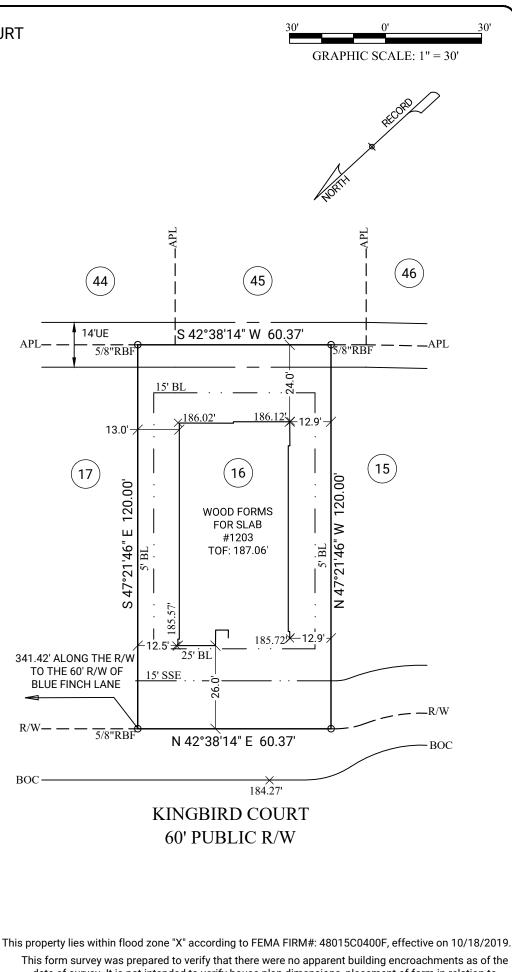
Approximate Property Line APL BOC Back of Curb R/W Right of Way N/F Now or Formerly UE **Utility Easement** Drainage Easement DF SSF Sanitary Sewer Easement WLE Water Line Easement STMSE Storm Sewer Easement PROP Proposed MFE **Minimum Finished Floor Elevation** FFF **Finished Floor Elevation** GFE **Garage Floor Elevation**
