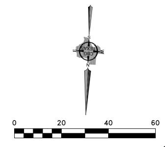
BEARINGS SHOWN ARE BASED ON NAD 83 TEXAS SOUTH CENTRAL ZONE. EASEMENTS AND BUILDING LINES ARE BY RECORDED PLAT UNLESS OTHERWISE
