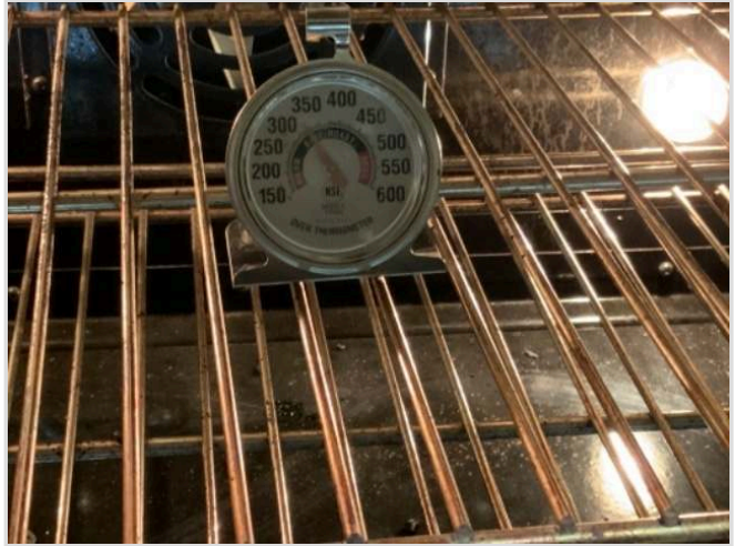
Thermometer showing 325 degrees (within tolerance)
